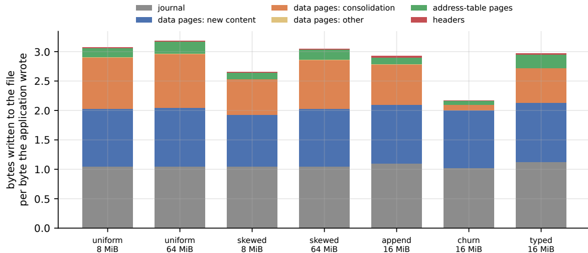
Figure 44.5: Where the bytes written to the file went, per byte the application wrote, over each whole run.
